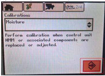
4. Make sure that grain tank is empty and engine is off! Use black thumb dial to highlight the white arrow and press checkmark button to go to next page.
