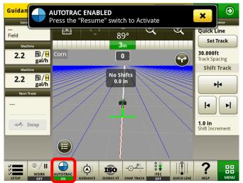
5. Press the "Auto" button right beside the throttle on the tractor to engage autotrac. Make sure you are close to your line before engaging autotrac.
