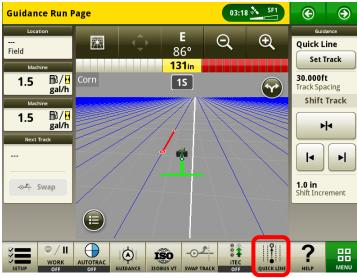
3. After pressing the "Quick Line" button drive 50 feet and the display will snap a line.
