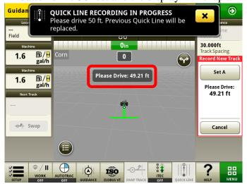
4. Once the vehicle has driven 50 feet the display will enable autotrac. Three out of four pieces of the autotrac pie will be filled in.
